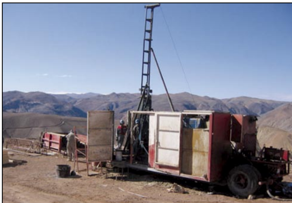
International PBX Ventures drills the Copaquire Projects' Sulfato Copper Zone as part of an aggressive drilling program to define a molybdenum-copper resource.
